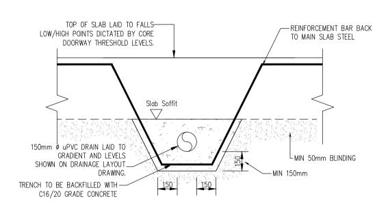
TYPICAL PIPE RUN TO SOFFIT OF SLAB
